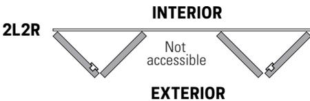
The above example (2L2R) is not recommended for interior applications because of the potential of getting locked in a room without any exit. Other configurations not recommended.
